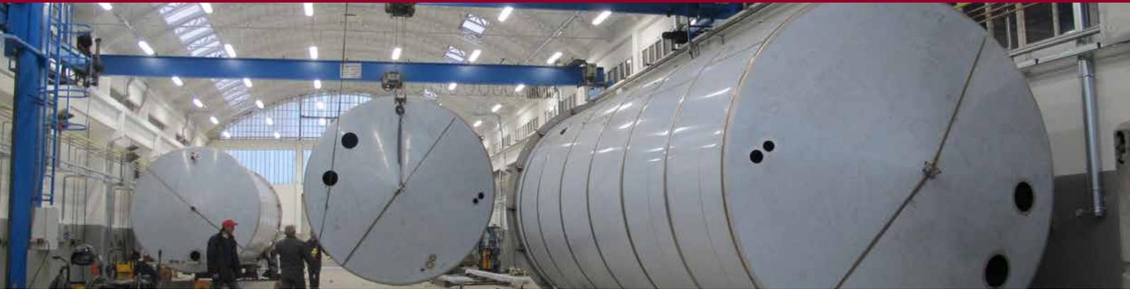
Vertical vessel in cylindrical form, single wall design.
